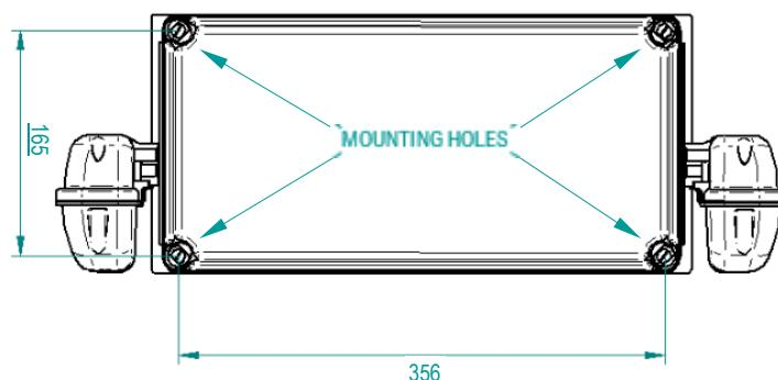
**Note:** This diagram shows the LWP2LIFE-PRO-WPOD in the wall mount configuration with the PODs rotated down. To mount to the ceiling using the same mounting instructions but ensure the heads are facing down
